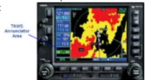
TAWS/Terrain Data Base Card Garmin GNS-530W with H-Taws
