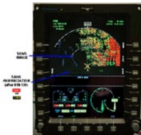
TAWS Display on MFD Map/Radar Page H-TAWS Displays "Under Glass"
